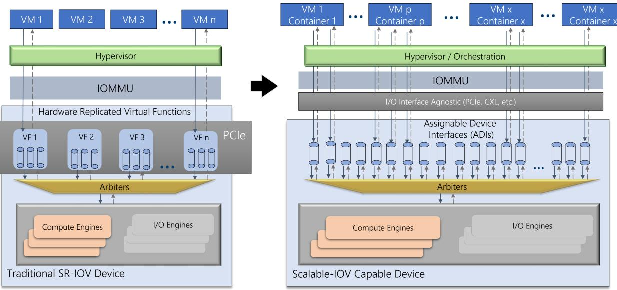
• While SR-IOV maps virtual devices as Virtual Functions (VFs) in HW, S-IOV composes virtual devices through light-weight and scalable Assignable Device Interfaces (ADIs) for fast-path operations and software mediated slow-path operations
