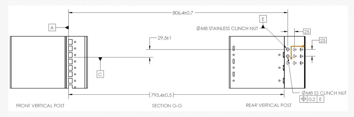
Start with Hole at Datum E and add holes to the busbar in a 25x25 array
