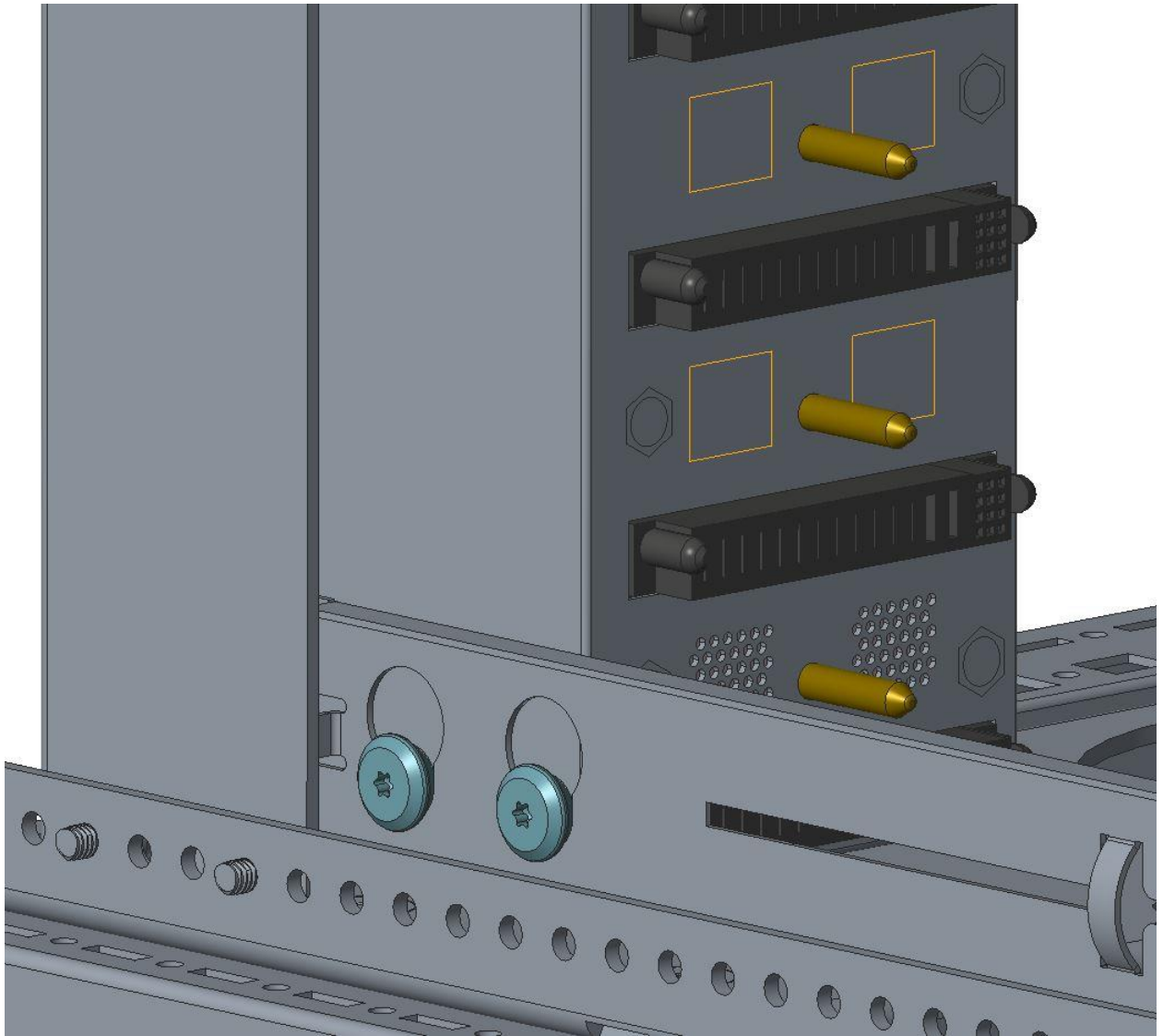
Figure 13. PMDU Rail Mounting: Inverted cone washers fit into keyhole slots in E2000 rails.
