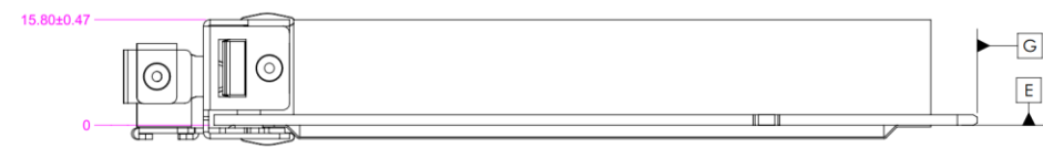
Figure 60: TSFF OCP NIC 3.0 Card with Ejector Latch CTF Dimensions (Top View)
