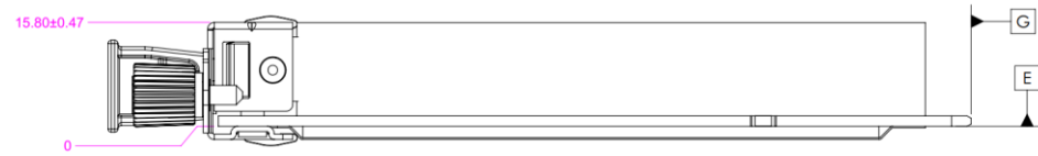
Figure 59: TSFF OCP NIC 3.0 Card with Pull Tab CTF Dimensions (Top View)
