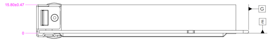
Figure 61: TSFF OCP NIC 3.0 Card with Internal Lock CTF Dimensions (Top View)
