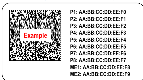
Figure 7263: MAC Address Label Example 2 – Octal Port with Single Host, Dual Managed Controller
