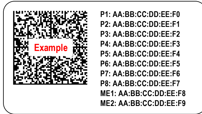
Figure 72: MAC Address Label Example 2 – Octal Port with Single Host, Dual Managed Controller
