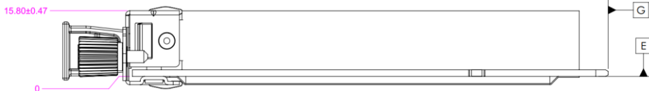
Figure 59: TSFF OCP NIC 3.0 Card with Pull Tab CTF Dimensions (Top View)
