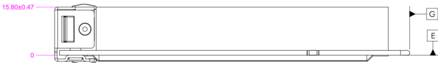
Figure 61: TSFF OCP NIC 3.0 Card with Internal Lock CTF Dimensions (Top View)
