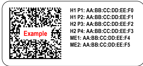
Figure 73: MAC Address Label Example 3 – Quad Port with Dual Hosts, Dual Managed Controllers
