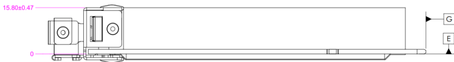
Figure 60: TSFF OCP NIC 3.0 Card with Ejector Latch CTF Dimensions (Top View)
