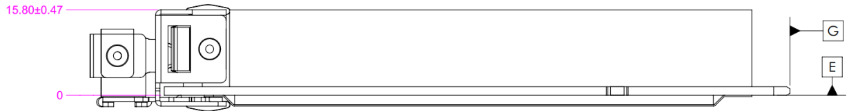
Figure 60: TSFF OCP NIC 3.0 Card with Ejector Latch CTF Dimensions (Top View)
