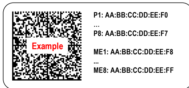
Figure 75: MAC Address Label Example 5 – Octal Port with Single Host, Octal Managed Controller
