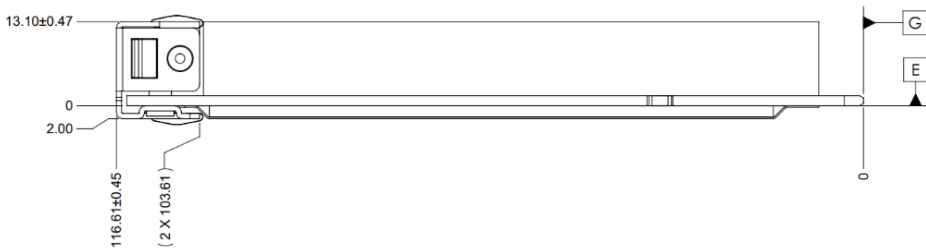
Figure 53: SFF OCP NIC 3.0 Card with Internal Lock CTF Dimensions (Side View)
