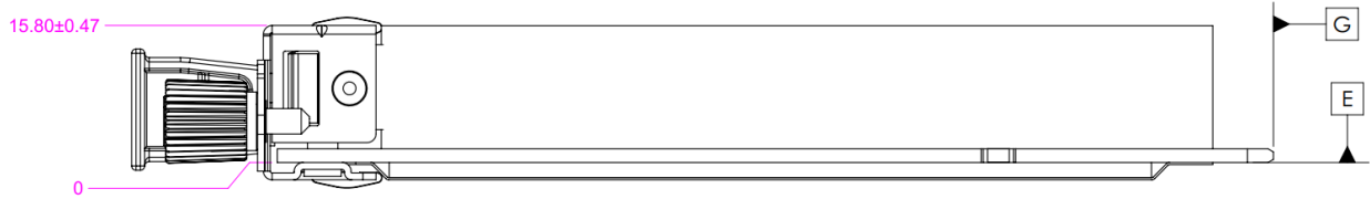
Figure 58: TSFF OCP NIC 3.0 Card with Pull Tab CTF Dimensions (Top View)
