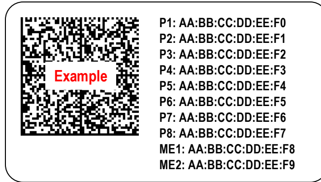
Figure 63: MAC Address Label Example 2 – Octal Port with Single Host, Dual Managed Controller
