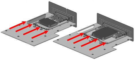
Figure <u>118</u>117: Airflow Direction for Hot Aisle Cooling (SFF and LFF)
