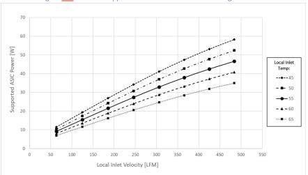
Figure <u>124</u>123: ASIC Supportable Power for Hot Aisle Cooling – LFF Card
