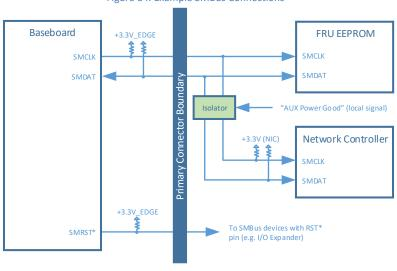
Figure 84: Example SMBus Connections
