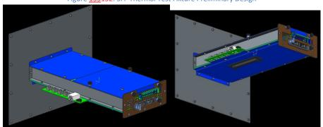
Figure <u>133</u>132: SFF Thermal Test Fixture Preliminary Design
