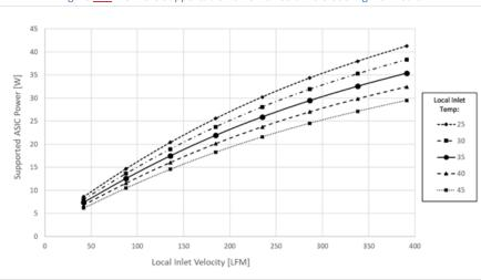
Figure  $\underline{\textbf{127}\textbf{126}}$ : ASIC Supportable Power for Cold Aisle Cooling – SFF Card
