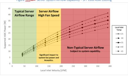
Figure <u>128</u><del>127</del>: Server System Airflow Capability – SFF Cold Aisle Cooling
