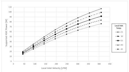
Figure 130129: ASIC Supportable Power for Cold Aisle Cooling – LFF Card
