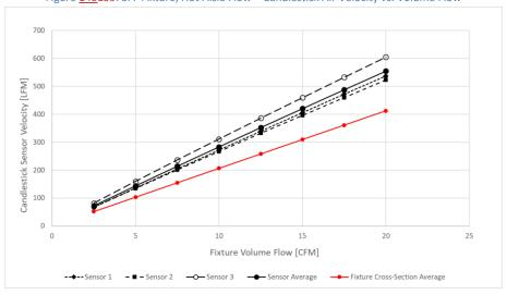
Figure <u>141140</u>: LFF Fixture, Hot Aisle Flow – Candlestick Air Velocity vs. Volume Flow
