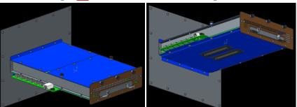
Figure <u>136</u>135: LFF Card Thermal Test Fixture Design
