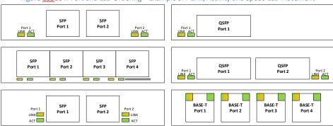
Note 1: The example port and LED ordering diagrams shown in Figure 105 Figure 104 are viewed with the card in the horizontal position and the primary side is facing up.
