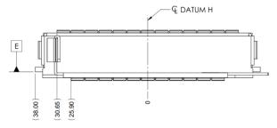
Figure 45: SFF OCP NIC 3.0 Card with Ejector CTF Dimensions (Side View)
