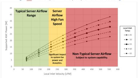
Figure 122121: Server System Airflow Capability – SFF Card Hot Aisle Cooling
