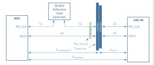
The following sections define the portion of the overall propagation delay budget allocated to the baseboard and to the OCP NIC 3.0 card, as well as additional requirements for each. Baseboard and NIC implementers shall analyze their design to ensure the timing budget is not violated.
