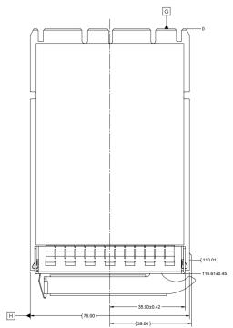
Figure 43: SFF OCP NIC 3.0 Card with Ejector CTF Dimensions (Top View)
