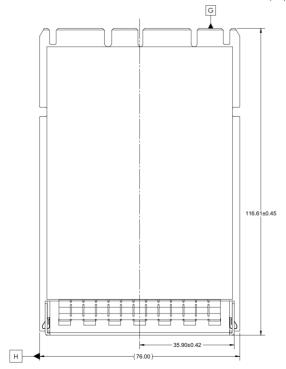
Figure 47: SFF OCP NIC 3.0 Card with Internal Lock CTF Dimensions (Front View)
