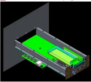
Figure <u>135</u>134: SFF Card Thermal Test Fixture PCB
