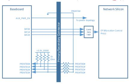
Figure 83: PCle Present and Bifurcation Control Pins (Static BIF[2:0:2]#)
