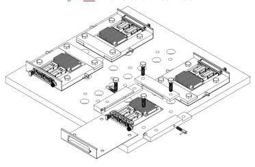
Figure <u>146</u>145: LFF Shock and Vibe Fixture
