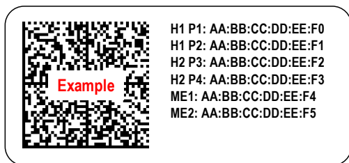
Figure 64: MAC Address Label Example 3 – Quad Port with Dual Hosts, Dual Managed Controllers
