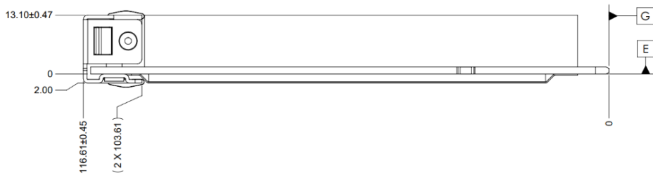
Figure 48: SFF OCP NIC 3.0 Card with Internal Lock CTF Dimensions (Side View)
