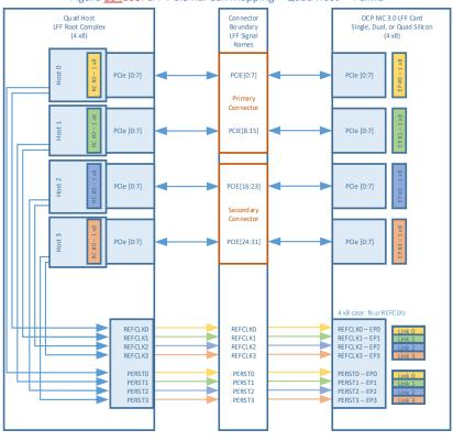
Figure 104103: LFF PCIe REFCLK Mapping – Quad Host – 4 Links
