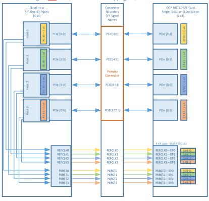
Figure 101100: SFF PCIe REFCLK Mapping – Quad Host – 4 Links
