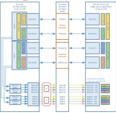
Figure 103102: LFF PCIe REFCLK Mapping – Dual Host – 2 and 4 links
