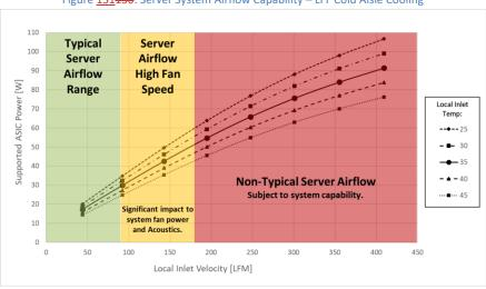
Figure <u>131</u>130: Server System Airflow Capability – LFF Cold Aisle Cooling
