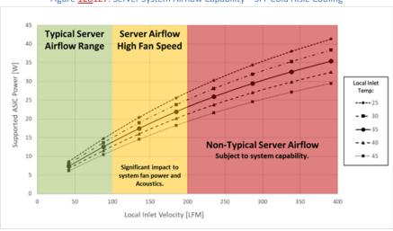
Figure <u>128</u><del>127</del>: Server System Airflow Capability – SFF Cold Aisle Cooling
