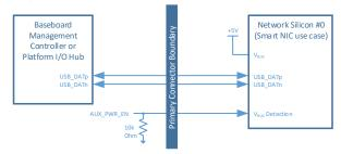
Figure <u>9291</u>: USB 2.0 Connection Example – USB-Serial / USB-JTAG Connectivity
