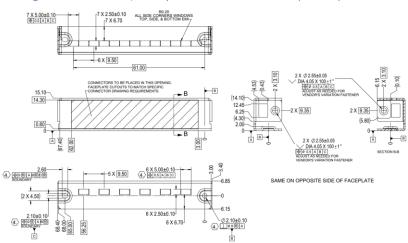
Figure 17: SFF Generic I/O Faceplate – Internal Lock Version (2D View)
