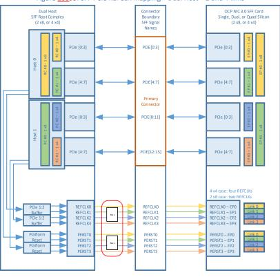
Figure 10099: SFF PCIe REFCLK Mapping – Dual Host – 2 and 4 links
