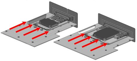
Figure 11817: Airflow Direction for Hot Aisle Cooling (SFF and LFF)
