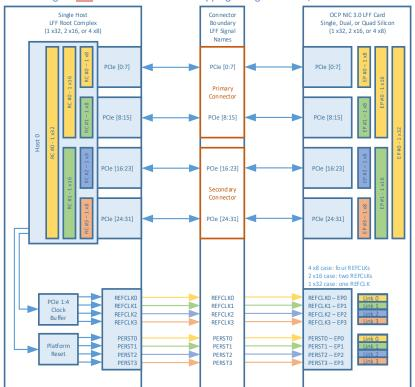
Figure 102101: LFF PCIe REFCLK Mapping – Single Host – 1, 2 and 4 links
