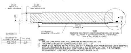
**Note:** The area defined by DIMENSION "A" is between the faceplate and the primary side of the board. Grounded through-hole mounting pins are permitted but should avoid making contact with the latching mechanism and EMI fingers. Signal pins are not permitted in this area.
