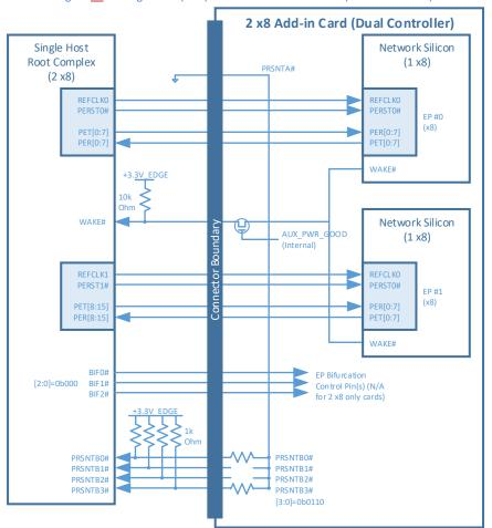
Figure 9594: Single Host (2 x8) and 2 x8 OCP NIC 3.0 Card (Dual Controllers)
