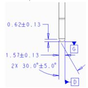
Figure 69: SFF Primary Conector Gold Finger - Detail D
