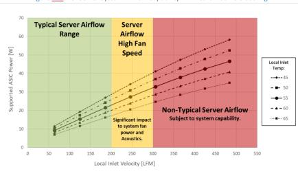
Figure <u>126</u>125: Server System Airflow Capability – LFF Card Hot Aisle Cooling
