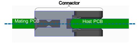
Figure 79: 0.3 mm Offset for 0.076" Thick Baseboards
