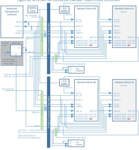
Figure 86: NC-SI over RBT Connection Example – Dual Primary Connectors
