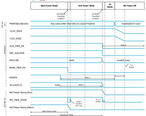
Figure <u>108</u>107: Power-Down Sequencing – Normal Operation
