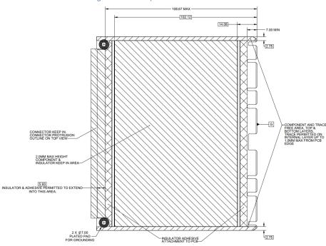
Figure 31: LFF Keep Out Zone – Bottom View
