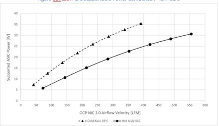
Figure <u>129</u>128: ASIC Supportable Power Comparison – SFF Card
