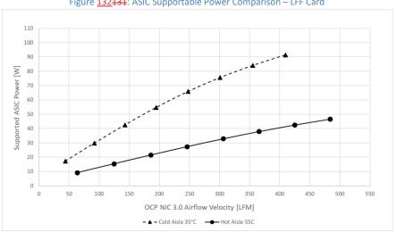
Figure <u>132</u>131: ASIC Supportable Power Comparison – LFF Card
