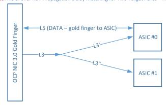
A clock buffer is optionally permitted if the NIC timing budget is not violated. This is shown in Figure 115Figure 114. In this case, the trace length would be calculated as the delay summation of trace segment L3 +  $T_{CLK_BUF}$  + L3' for ASIC #0, and L3 +  $T_{CLK_BUF}$  + L3' for ASIC #1.
