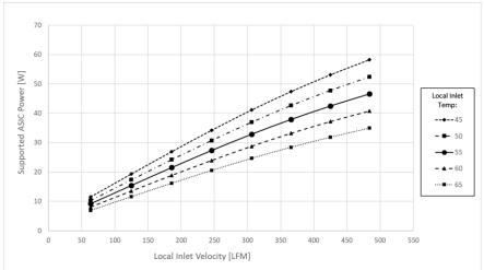
Figure <u>124123</u>: ASIC Supportable Power for Hot Aisle Cooling – LFF Card
