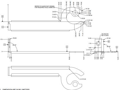
Figure 19: SFF I/O Faceplate – Ejector Lever (2D View)
