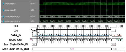
Figure 88: Scan Chain Timing Diagram Example 2
