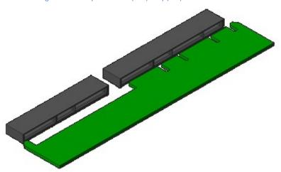
For both form factors, an OCP NIC 3.0 card may optionally implement a subset of pins to support less than a x16 PCIe connection. This may be implemented using a 2C+ card edge per SFF-TA-1002. The baseboard Primary Connector shall use a 4C+ in all cases. Figure 6 illustrates the supported 4C+ and 2C+ card edge configurations on a 4C+ Primary Connector.
