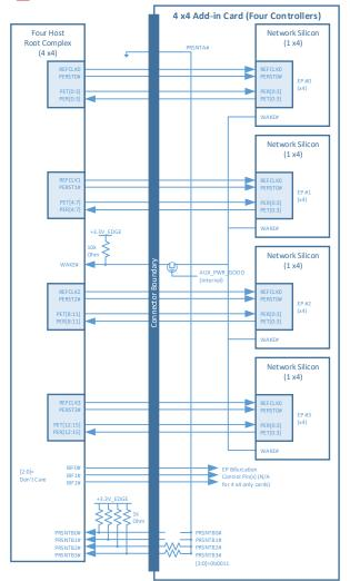
Figure 9796: Quad Hosts (4 x4) and 4 x4 OCP NIC 3.0 Card (Quad Controllers)
