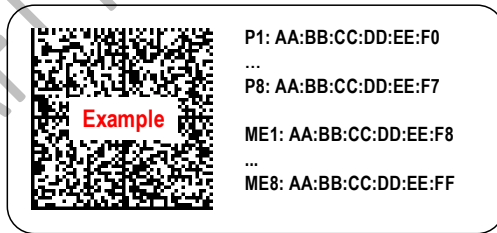
Figure 66: MAC Address Label Example 5 – Octal Port with Single Host, Octal Managed Controller
