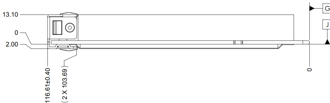
Figure 48: SFF OCP NIC 3.0 Card with Internal Lock CTF Dimensions (Side View)
