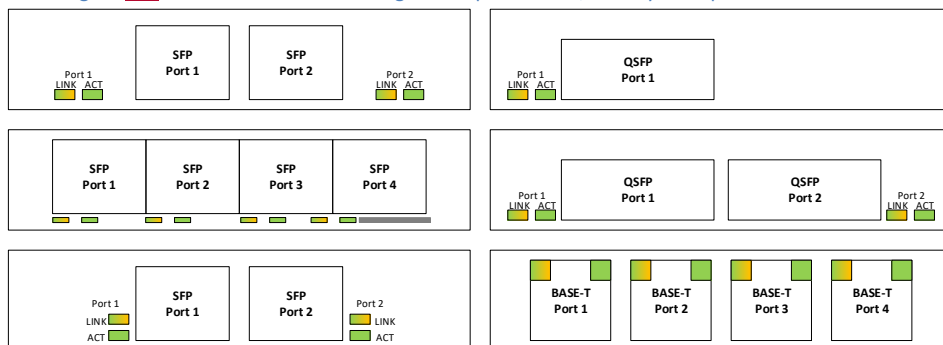
Figure 104103: Port and LED Ordering – Example SFF Link/Activity and Speed LED Placement
