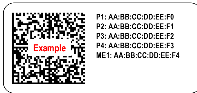
Figure 62: MAC Address Label Example 1 – Quad Port with Single Host, Single Managed Controller
