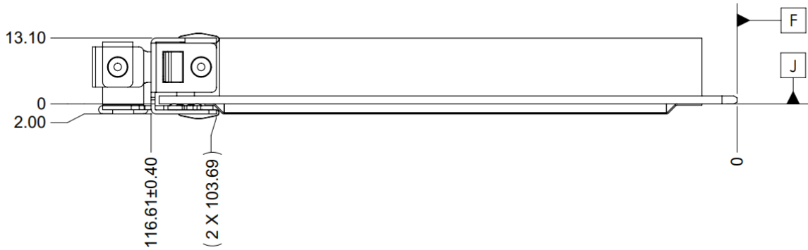
Figure 56: LFF OCP NIC 3.0 Card with Ejector CTF Dimensions (Side View)
