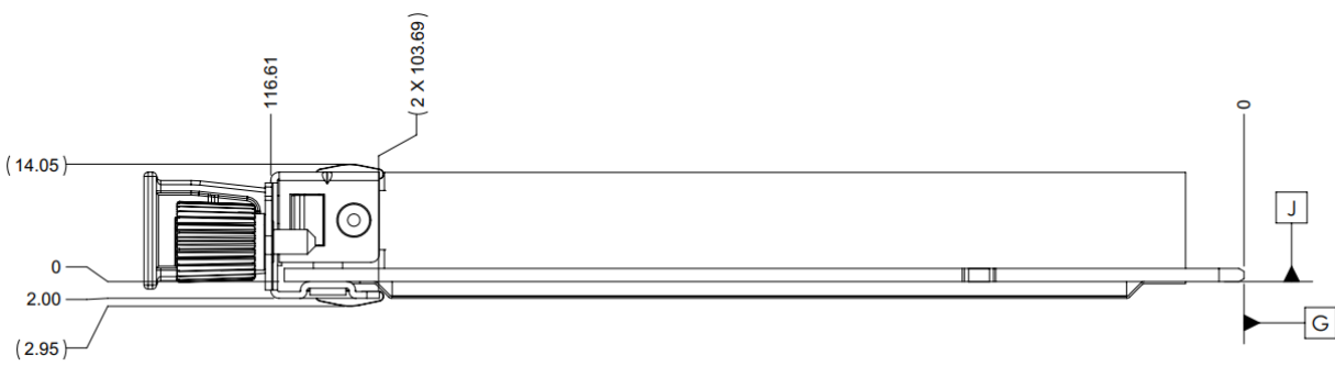
Figure 42: SFF OCP NIC 3.0 Card with Pull Tab CTF Dimensions (Side View)
