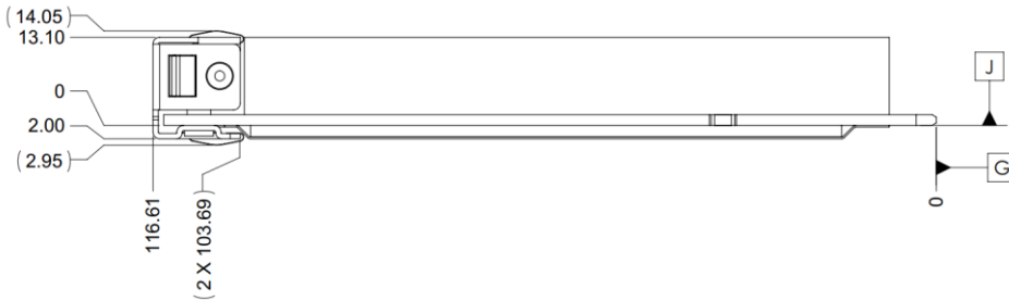
Figure 48: SFF OCP NIC 3.0 Card with Internal Lock CTF Dimensions (Side View)
