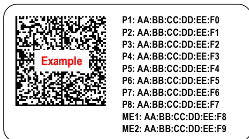
Figure 63: MAC Address Label Example 2 – Octal Port with Single Host, Dual Managed Controller
