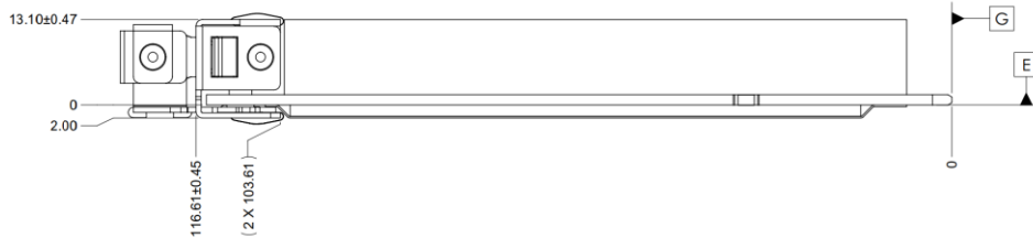
Figure 45: SFF OCP NIC 3.0 Card with Ejector CTF Dimensions (Side View)
