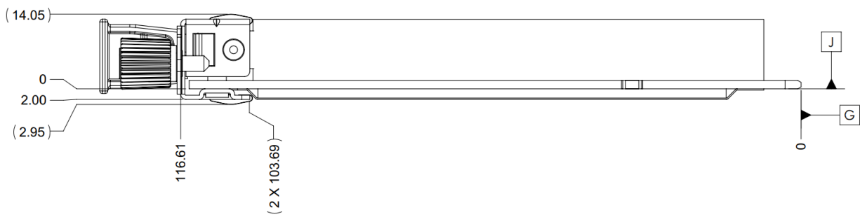
Figure 42: SFF OCP NIC 3.0 Card with Pull Tab CTF Dimensions (Side View)
