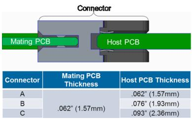
The connectors are capable of being used coplanar as shown in Figure 77. Additionally, the connectors are also capable of having a 0.3 mm offset from the centerline of the host board as shown in Figure 78.
