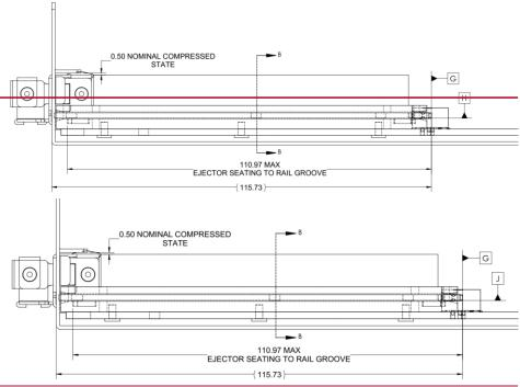
Figure 59: LFF Baseboard Chassis CTF Dimensions (Rail Guide View)
