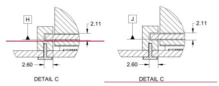
The right angle and straddle mount card guides are identical between the SFF and LFF. The card guide models are included in the 3D CAD packages and may be downloaded from the OCP NIC 3.0 Wiki site: <a href="http://www.opencompute.org/wiki/Server/Mezz">http://www.opencompute.org/wiki/Server/Mezz</a>.
