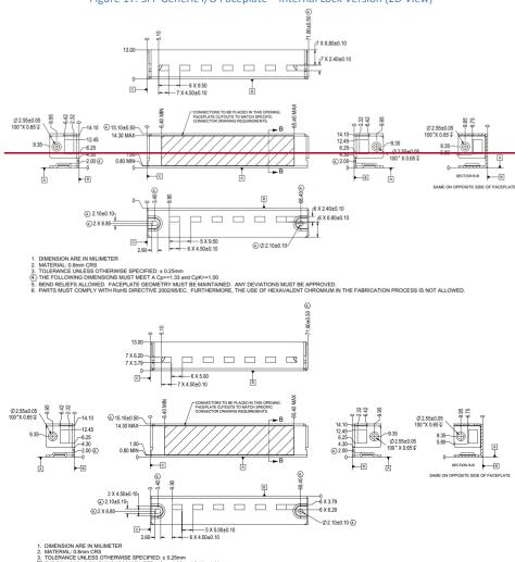
Figure 17: SFF Generic I/O Faceplate – Internal Lock Version (2D View)
