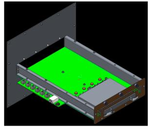
Figure 129: LFF Card Thermal Test Fixture PCB
