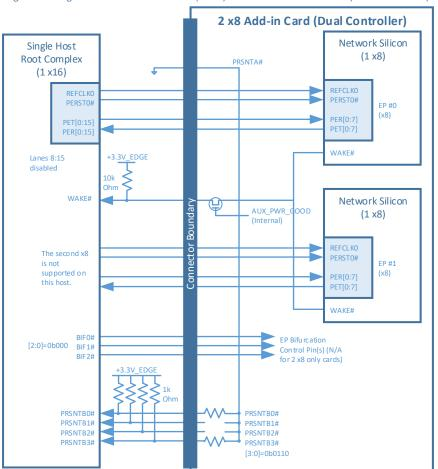
Figure 96: Single Host with no Bifurcation (1 x16) and 2 x8 OCP NIC 3.0 Card (Dual Controllers)
