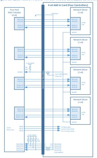
Figure 95: Quad Hosts (4 x4) and 4 x4 OCP NIC 3.0 Card (Quad Controllers)
