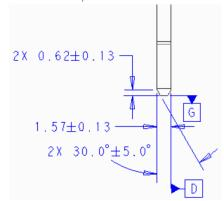
Figure 68: SFF Primary Conector Gold Finger - Detail D
