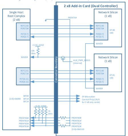
Figure 93: Single Host (2 x8) and 2 x8 OCP NIC 3.0 Card (Dual Controllers)
