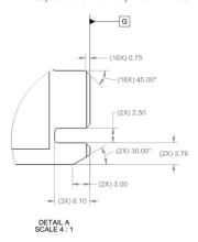
Figure 31: LFF Keep Out Zone – Bottom View
