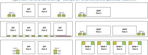
Note 1: The example port and LED ordering diagrams shown in Figure 103 are viewed with the card in the horizontal position and the primary side is facing up.
