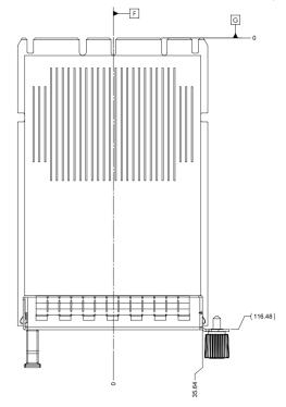
Figure 41: SFF OCP NIC 3.0 Card with Pull Tab CTF Dimensions (Front View)
