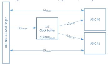
Figure 107: NC-SI over RBT Propagation Delay Matching
