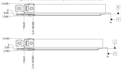
Figure 56: LFF OCP NIC 3.0 Card with Ejector CTF Dimensions (Side View)
