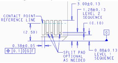
Figure 69: LFF Gold Finger Dimensions – x32 – Top Side ("B" Pins)
