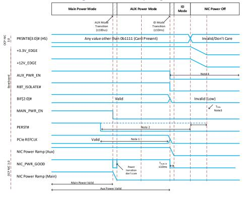
Figure 106: Power-Down Sequencing
