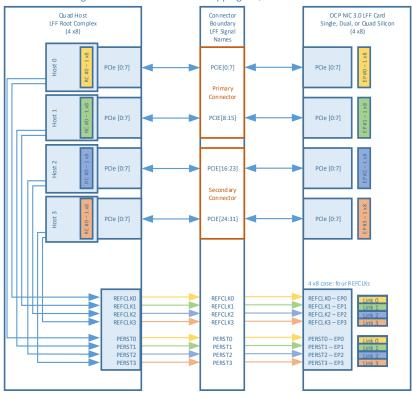
Figure 102: LFF PCIe REFCLK Mapping – Quad Host – 4 Links
