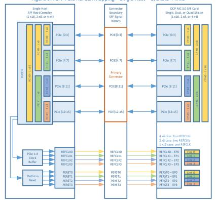
Figure 97: SFF PCIe REFCLK Mapping – Single Host – 1, 2 and 4 links
