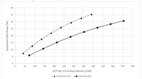
Figure 120: ASIC Supportable Power Comparison – SFF Card
