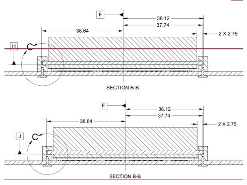
Figure 53: SFF Baseboard Chassis CTF Dimensions (Rail Guide Detail) – Detail C
