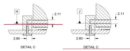
The right angle and straddle mount card guides are identical between the SFF and LFF cards. The card guide model is included in the 3D CAD packages and may be downloaded from the OCP NIC 3.0 Wiki site: <a href="http://www.opencompute.org/wiki/Server/Mezz">http://www.opencompute.org/wiki/Server/Mezz</a>.
