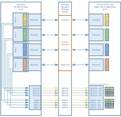
Figure 99: SFF PCIe REFCLK Mapping – Quad Host – 4 Links
