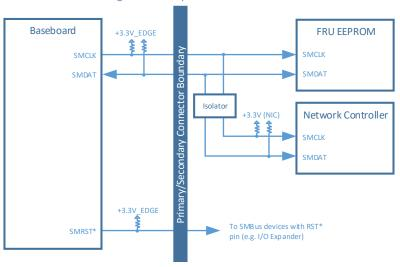
Figure 83: Example SMBus Connections
