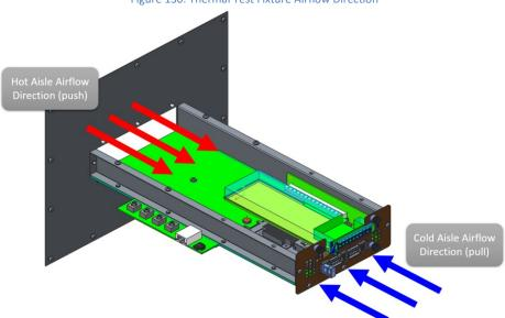
Figure 130: Thermal Test Fixture Airflow Direction
