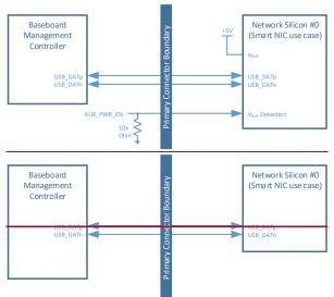
Figure 89: USB 2.0 Connection Example – Basic Connectivity
