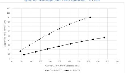
Figure 123: ASIC Supportable Power Comparison – LFF Card
