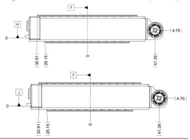
Figure 42: SFF OCP NIC 3.0 Card with Pull Tab CTF Dimensions (Side View)
