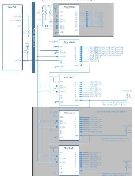
Figure 87: Scan Chain Connection Example
