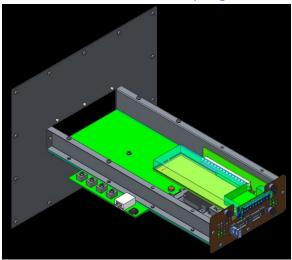
Figure 126: SFF Card Thermal Test Fixture PCB
