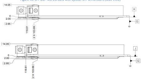
Figure 45: SFF OCP NIC 3.0 Card with Ejector CTF Dimensions (Side View)
