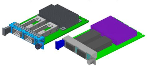
Figure 113: OCP NIC 3.0 SFF Reference Design and CFD Geometry
