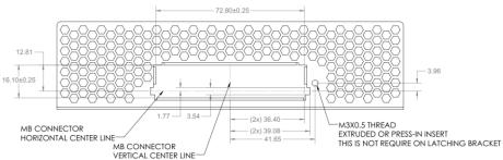
Figure 49: SFF Baseboard Chassis CTF Dimensions (Rear View)
