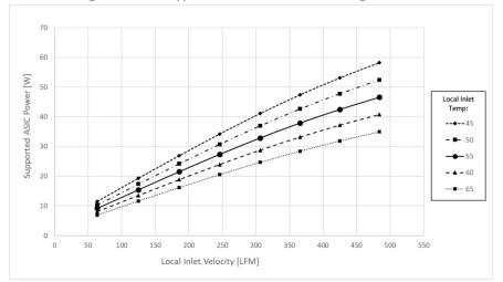
Figure 115: ASIC Supportable Power for Hot Aisle Cooling – LFF Card
