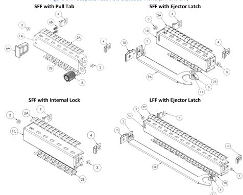
Figure 14: Faceplate Assembly Exploded Views (SFF and LFF)
