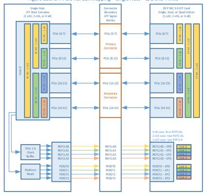
Figure 100: LFF PCIe REFCLK Mapping – Single Host – 1, 2 and 4 links
