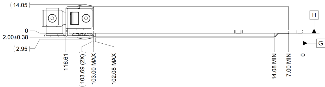
Figure 53: LFF OCP NIC 3.0 Card with Ejector CTF Dimensions (Side View)
