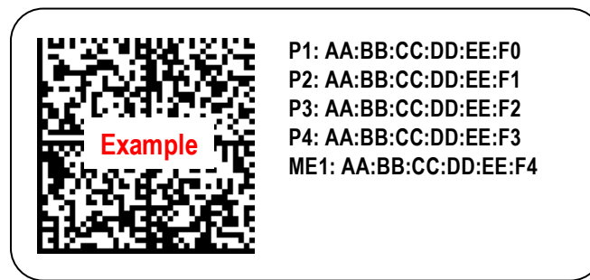
Figure 59: MAC Address Label Example 1 – Quad Port with Single Host, Single Managed Controller
