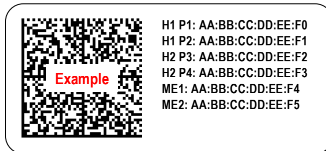
Figure 61: MAC Address Label Example 3 – Quad Port with Dual Hosts, Dual Managed Controllers
