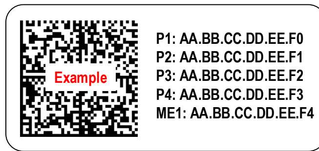
Figure 57: MAC Address Label Example 1 – Quad Port with Single Host, Single Managed Controller
