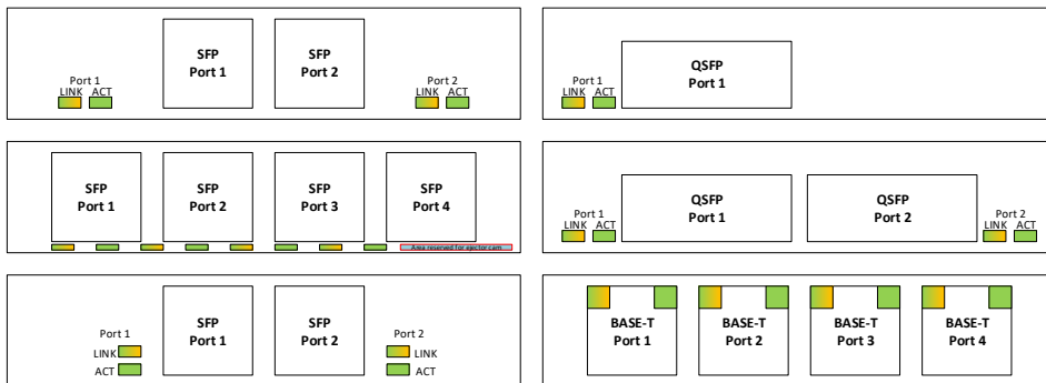
Figure 92: Port and LED Ordering – Example SFF Link/Activity and Speed LED Placement
