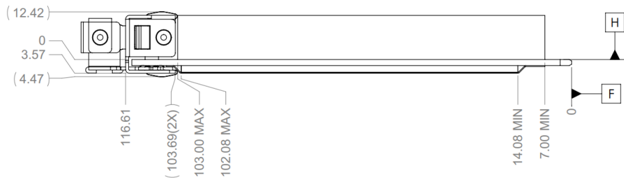
Figure 51: LFF OCP NIC 3.0 Card with Ejector CTF Dimensions (Side View)
