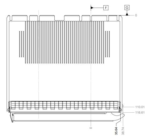
Figure 49: LFF OCP NIC 3.0 Card with Ejector CTF Dimensions (Top View)
