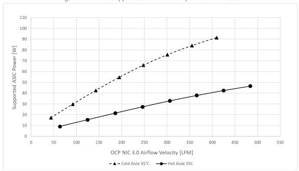
Figure 111: ASIC Supportable Power Comparison – LFF Card
