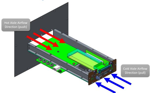
Figure 118: Thermal Test Fixture Airflow Direction
