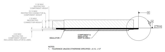
Figure 32: LFF Keep Out Zone – Side View
