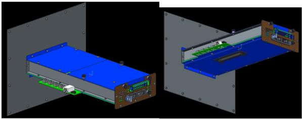
Figure 112: SFF Thermal Test Fixture Preliminary Design
