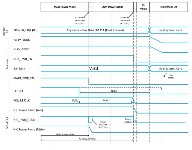
Figure 95: Power-Down Sequencing
