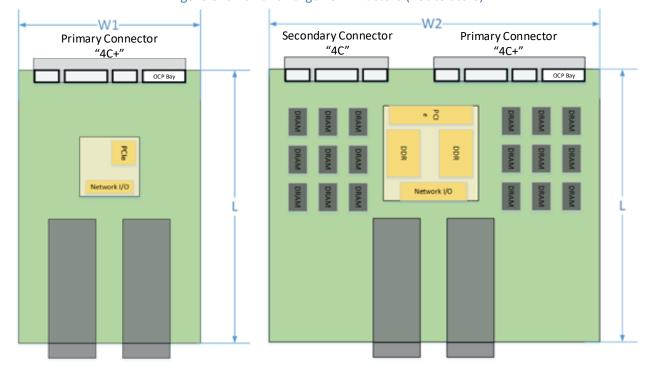
Figure 3: Small and Large Form-Factors (not to scale)
