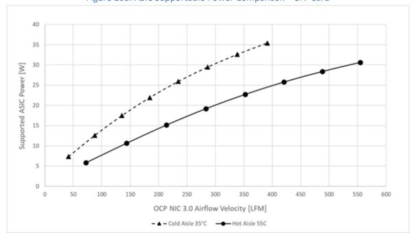
Figure 108: ASIC Supportable Power Comparison – SFF Card
