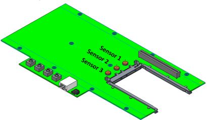
Figure 114: SFF Card Thermal Test Fixture PCB
