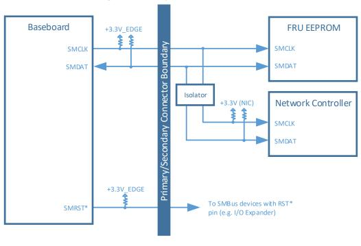
Figure 76: Example SMBus Connections
