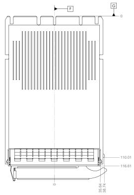
Figure 41: SFF OCP NIC 3.0 Card with Ejector CTF Dimensions (Top View)
