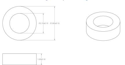
Figure 22: Ejector Bushing
