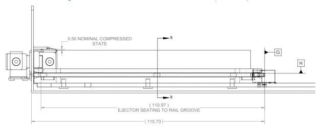
Figure 53: LFF Baseboard Chassis CTF Dimensions (Side View)
