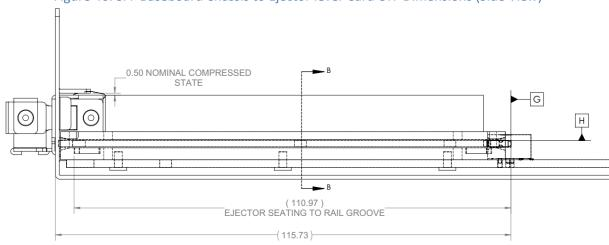
Figure 46: SFF Baseboard Chassis to Ejector lever Card CTF Dimensions (Side View)
