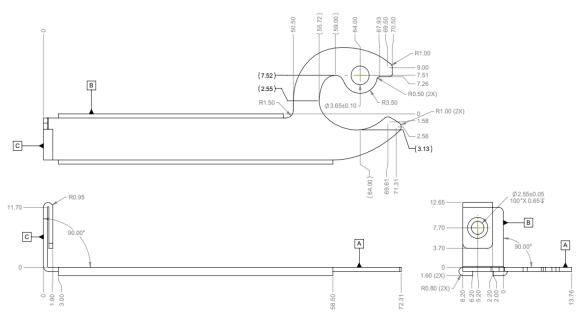
Figure 19: SFF I/O Faceplate – Ejector Lever (2D View)
