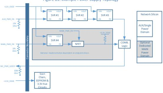
Figure 81: Example Power Supply Topology
