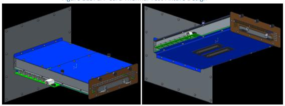
Figure 115: LFF Card Thermal Test Fixture Design
