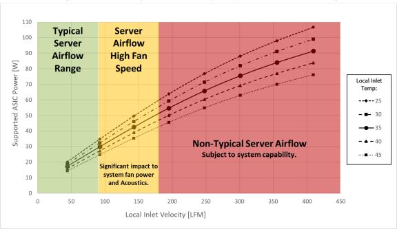
Figure 110: Server System Airflow Capability – LFF Cold Aisle Cooling
