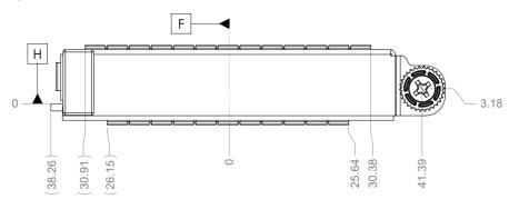
Figure 39: SFF OCP NIC 3.0 Card with Pull Tab CTF Dimensions (Front View)
