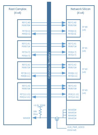
Figure 91: PCIe Interface Connections for a 4 x4 OCP NIC 3.0 Card
