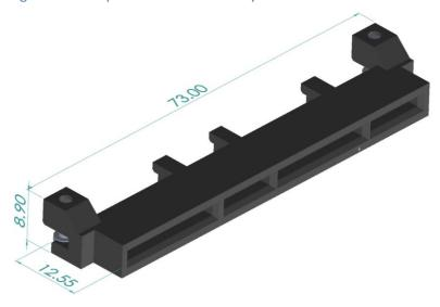
Figure 68: 140-pin Base Board Secondary Connector – Straddle Mount
