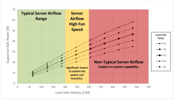
Figure 105: Server System Airflow Capability – LFF Card Hot Aisle Cooling
