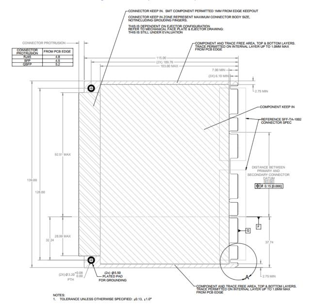
Figure 29: LFF Keep Out Zone - Top View
