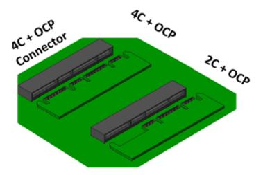
Table 5 summarizes the supported card form factors. Small form factor cards support the Primary Connector and up to 16 PCle lanes. Large form factor cards support implementations with both the Primary and Secondary Connectors and up to 32 PCle lanes, or a Primary Connector only implementation with up to 16 PCle lanes.
