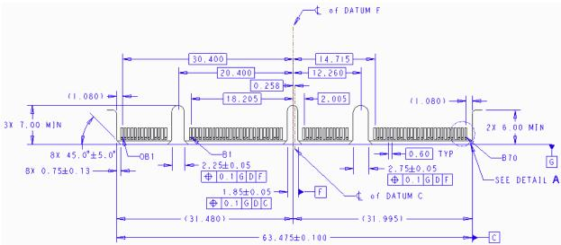
Figure 61: SFF Primary Connector Gold Finger Dimensions – x16 – Top Side ("B" Pins)
