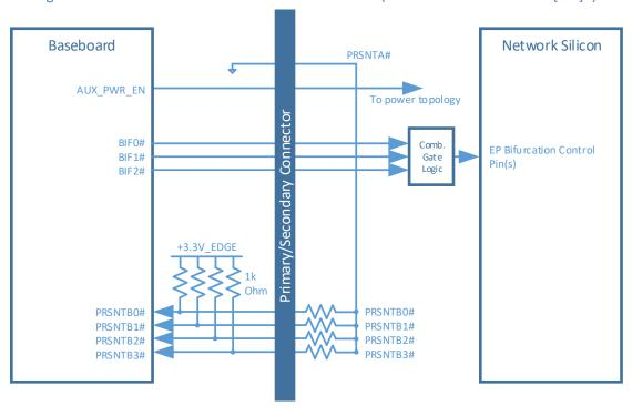
Figure 74: PCIe Present and Bifurcation Control Pins (Baseboard Controlled BIF[0:2]#)
