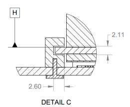
The right angle and straddle mount card guides are identical between the Small and Large form factor cards. The card guide model is included in the 3D CAD packages and may be downloaded from the OCP NIC 3.0 Wiki site: <a href="http://www.opencompute.org/wiki/Server/Mezz">http://www.opencompute.org/wiki/Server/Mezz</a>.
