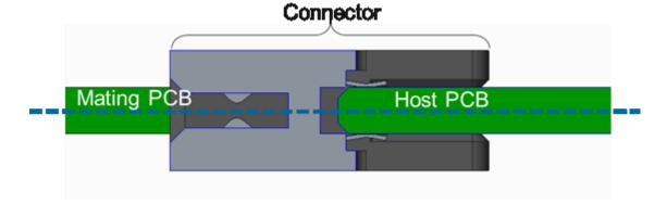
Figure 70: 0mm Offset (Coplanar) for 0.062" Thick Baseboards
