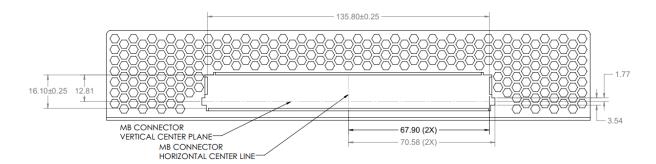
Figure 52: LFF Baseboard Chassis CTF Dimensions (Rear View)
