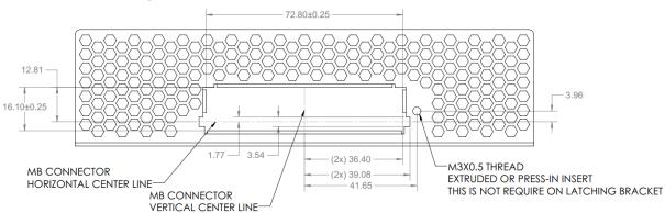
Figure 44: SFF Baseboard Chassis CTF Dimensions (Rear View)
