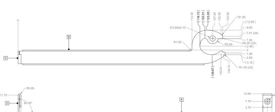
Figure 20: LFF I/O Faceplate – Ejector Lever (2D View)
