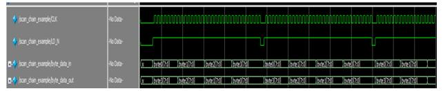
The scan chain provides sideband status indication between the OCP NIC 3.0 card and the baseboard. The scan chain bit definition is defined in the two tables below. The scan chain data stream is 32-bits in length for both the DATA\_OUT and the DATA\_IN streams. The scan chain implementation is optional on
