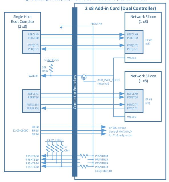
Figure 86: Single Host (2 x8) and 2 x8 OCP NIC 3.0 Card (Dual Controllers)
