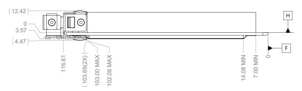
Figure 51: LFF OCP NIC 3.0 Card with Ejector CTF Dimensions (Side View)
