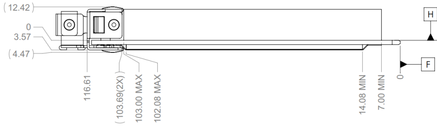
Figure 51: Large Form Factor LFF OCP NIC 3.0 Card with Ejector CTF Dimensions (Side View)
