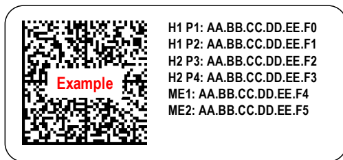
Figure 59: MAC Address Label Example 3 – Quad Port with Dual Hosts, Dual Managed Controllers
