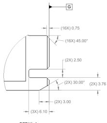
Figure 30: Large Form Factor Keep Out Zone – Top View – Detail A
