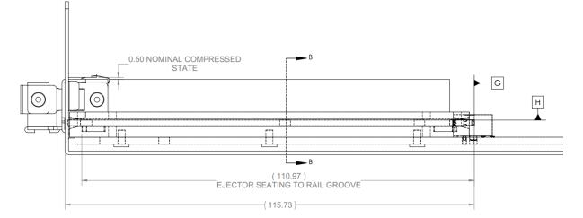
Figure 53: Large Form Factor Baseboard Chassis CTF Dimensions (Side View)
