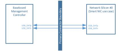
Figure 83: USB 2.0 Connection Example – USB-Serial / USB-JTAG Connectivity
