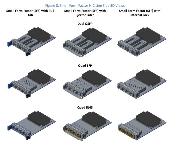
Figure 9 illustrates example SFF 3D views of the pull tab and ejector latch assemblies mounted in a chassis utilizing a straddle mount connector and a right angle connector. The baseboard connector options are discussed in Section 3.2. The SFF OCP NIC 3.0 card is identical for both chassis connector options.
