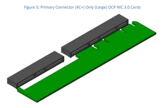
For both form-factors, an OCP NIC 3.0 card may optionally implement a subset of pins to support less than a x16 PCIe connection. This may be implemented using a 2C+ card edge per SFF-TA-1002. The baseboard Primary Connector shall use a 4C+ in all cases. Figure 6 illustrates the supported 4C+ and 2C+ card edge configurations on a 4C+ Primary Connector.
