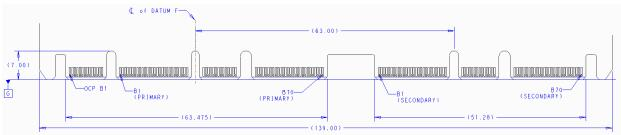
Figure 62: Large Size Card Gold Finger Dimensions – x32 – Top Side ("B" Pins)
