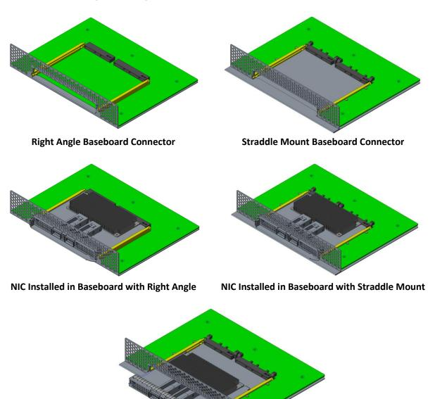
Figure 12: Large Form Factor NIC Chassis Mounted 3D Views
