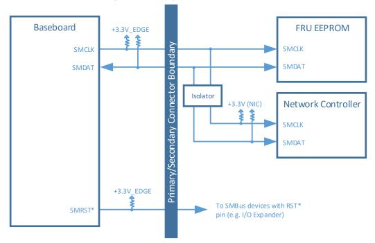
Figure 76: Example SMBus Connections
