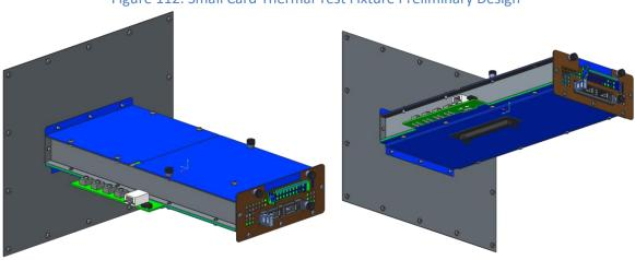
Figure 112: Small Card Thermal Test Fixture Preliminary Design
