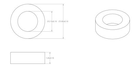
DIMENSION ARE IN MILIMETER MATERIAL: STEEL SAE 1215 TOLERANCE UNLESS OTHERWISE SPECIFIED: ± 0.25mm, ±1.0° PARTS MUST COMPLY WITH RoHS DIRECTIVE 2002/95/EC. FURTHERMORE, THE USE OF HEXAVALENT CHROMIUM IN THE FABRICATION PROCESS IS NOT ALLOWED. 1. 2. 3. 4.
