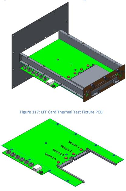
Figure 116: LFF Card Thermal Test Fixture Design – Cover Removed
