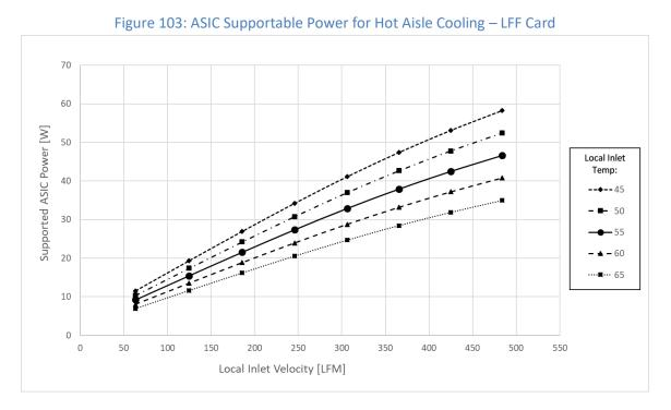
The curves shown in Figure 103 were obtained using CFD analysis of the reference OCP NIC 3.0 LFF card. The reference card has a 45mm x 45mm ASIC with two QSFP connectors. Additional card geometry parameters and boundary conditions used in the reference CFD analysis are summarized in Table 66. Figure 104 shows a comparison of the 3D CAD and CFD model geometry for the reference OCP NIC 3.0 card.
