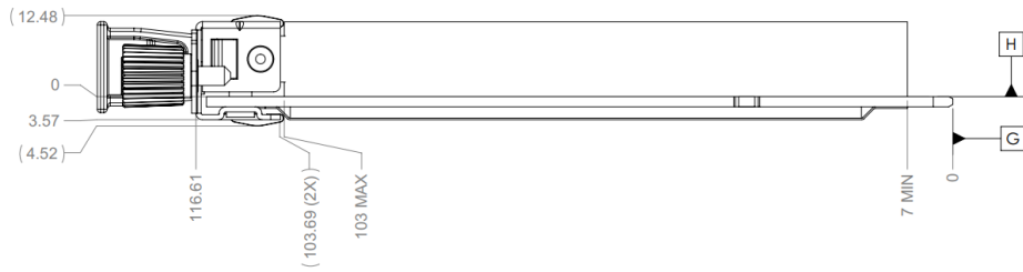
Figure 40: Small Form Factor OCP NIC 3.0 Card with Pull Tab CTF Dimensions (Side View)
