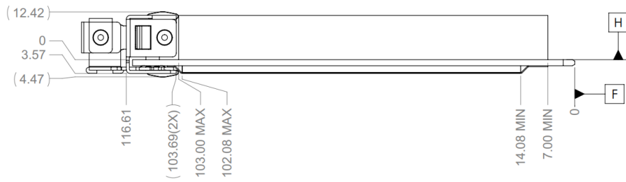
Figure 51: Large Form Factor OCP NIC 3.0 Card with Ejector CTF Dimensions (Side View)
