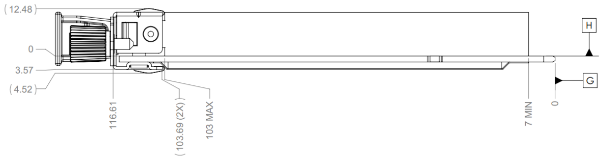
Figure 40: Small Form Factor OCP NIC 3.0 Card with Pull Tab CTF Dimensions (Side View)
