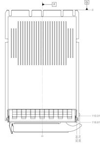
Figure 42: Small Form Factor OCP NIC 3.0 Card with Ejector CTF Dimensions (Front View)
