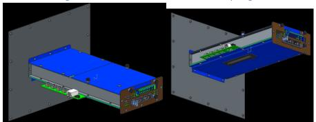
Figure 107: Small Card Thermal Test Fixture Preliminary Design
