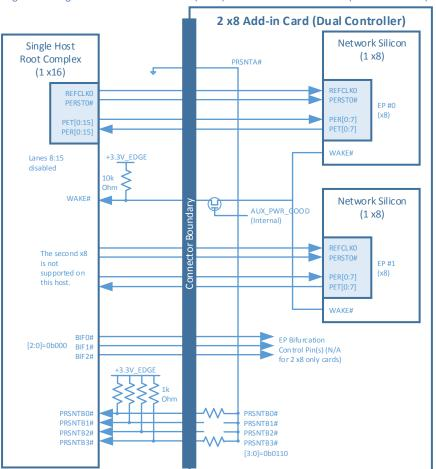
Figure 86: Single Host with no Bifurcation (1 x16) and 2 x8 OCP NIC 3.0 Card (Dual Controllers)
