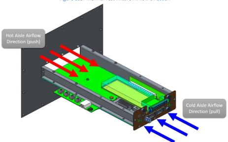
Figure 113: Thermal Test Fixture Airflow Direction
