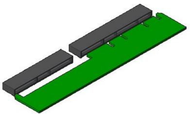
For both form-factors, an OCP NIC 3.0 card may optionally implement a subset of pins to support up to a x8 PCle connection. This is implemented using a 2C card edge per SFF-TA-1002. The Primary Connector may support a 2C sized OCP NIC 3.0 card along with the 28 pin OCP bay shown in the 4C+ drawings. The following diagram from the SFF-TA-1002 specification illustrates the supported host Primary and Secondary Connectors and OCP NIC 3.0 card configurations.
