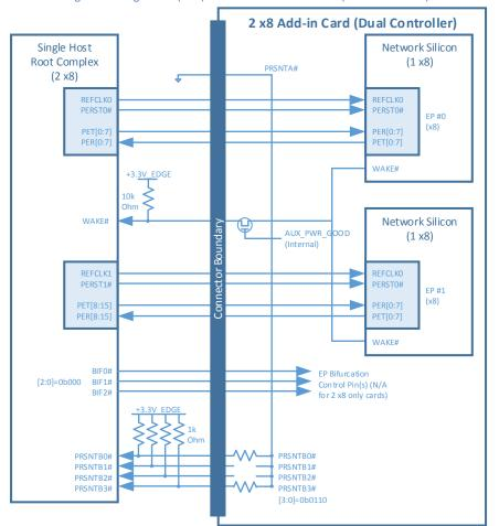
Figure 83: Single Host (2 x8) and 2 x8 OCP NIC 3.0 Card (Dual Controllers)
