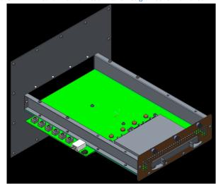
Figure 112: LFF Card Thermal Test Fixture PCB
