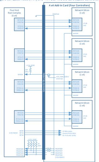
Figure 85: Quad Hosts (4 x4) and 4 x4 OCP NIC 3.0 Card (Quad Controllers)
