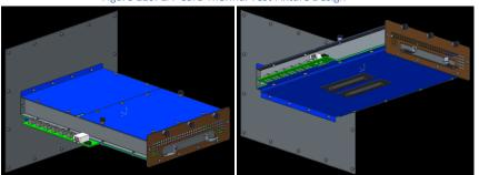
Figure 110: LFF Card Thermal Test Fixture Design
