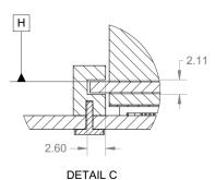
The right angle and straddle mount card guides are identical between the Small and Large form factor cards. The card guide models are included in the 3D CAD packages and may be downloaded from the OCP NIC 3.0 Wiki site: <a href="http://www.opencompute.org/wiki/Server/Mezz">http://www.opencompute.org/wiki/Server/Mezz</a>.
