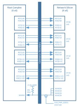
Figure 88: PCIe Interface Connections for a 4 x4 OCP NIC 3.0 Card
