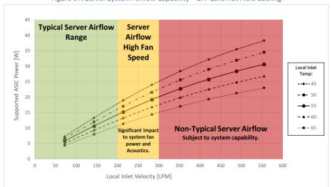
Figure 97: Server System Airflow Capability – SFF Card Hot Aisle Cooling
