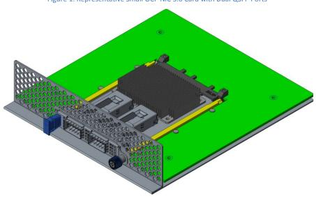
Figure 1: Representative Small OCP NIC 3.0 Card with Dual QSFP Ports
