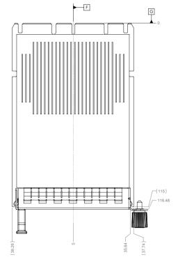
Figure 39: Small Form Factor OCP NIC 3.0 Card with Pull Tab CTF Dimensions (Front View)
