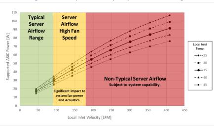
Figure 105: Server System Airflow Capability – LFF Cold Aisle Cooling
