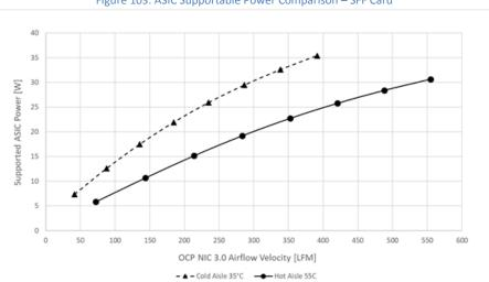
Figure 103: ASIC Supportable Power Comparison – SFF Card
