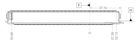
Figure 51: Large Form Factor OCP NIC 3.0 Card with Ejector CTF Dimensions (Side View)
