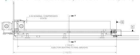
Figure 47: Small Form Factor Baseboard Chassis CTF Dimensions (Rear Rail Guide View)
