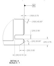
Figure 31: Large Form Factor Keep Out Zone – Bottom View
