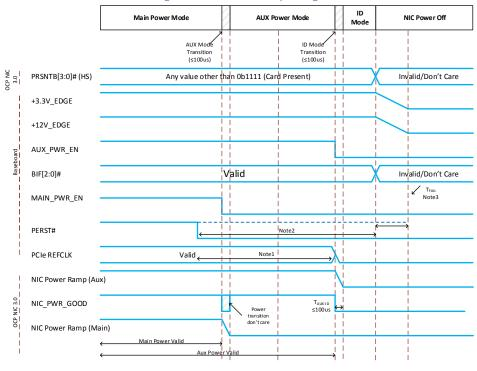
Figure 92: Power-Down Sequencing
