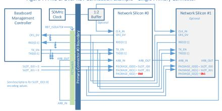
Figure 77: NC-SI Over RBT Connection Example – Single Primary Connector
