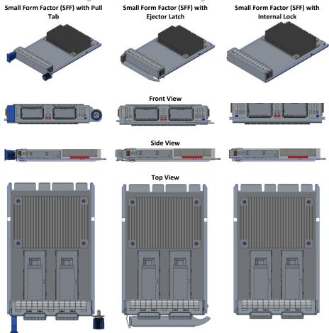
Figure 8 illustrates example SFF 3D views for the supported line side I/O implementations. The line side I/O implementations are discussed in Section 2.2.
