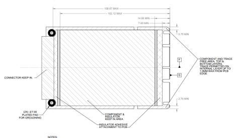
Figure 26: Small Form Factor Keep Out Zone – Bottom View
