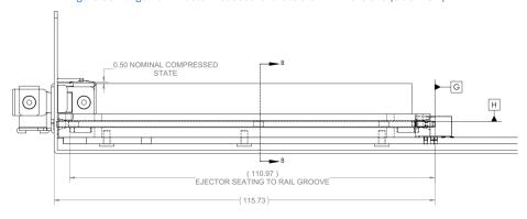
Figure 54: Large Form Factor Baseboard Chassis CTF Dimensions (Rail Guide View)
