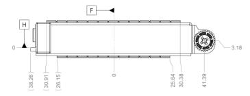
Figure 40: Small Form Factor OCP NIC 3.0 Card with Pull Tab CTF Dimensions (Side View)
