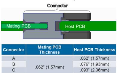
The connectors are capable of being used coplanar as shown in Figure 70. Additionally, the connectors are also capable of having a 0.3mm offset from the centerline of the host board as shown in Figure 71.
