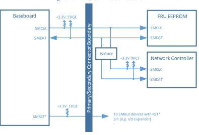
Figure 76: Example SMBus Connections
