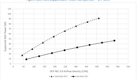
Figure 106: ASIC Supportable Power Comparison – LFF Card
