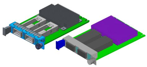
Figure 96: OCP NIC 3.0 SFF Reference Design and CFD Geometry
