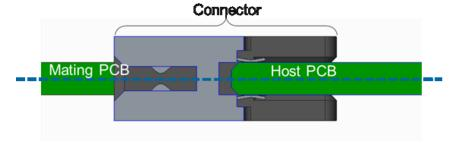
Figure 71: 0.3mm Offset for 0.076" Thick Baseboards
