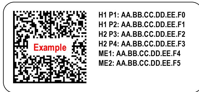
Figure 57: MAC Address Label Example 3 – Quad Port with Dual Hosts, Dual Managed Controllers
