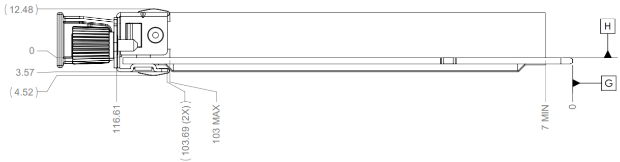
Figure 38: Small Form Factor OCP NIC 3.0 Card with Pull Tab CTF Dimensions (Side View)
