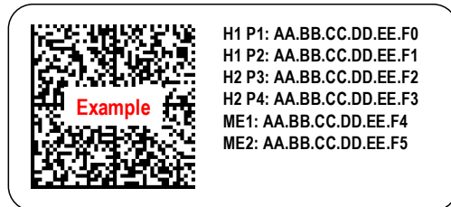
Figure 57: MAC Address Label Example 3 – Quad Port with Dual Hosts, Dual Managed Controllers
