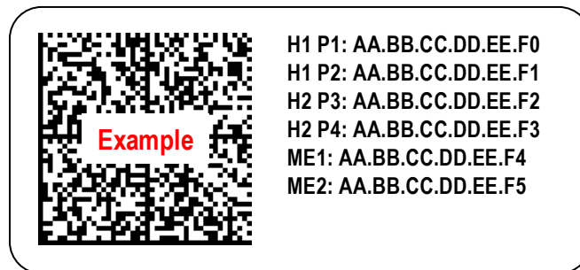
Figure 58: MAC Address Label Example 3 – Dual Host, Quad Port, Single Managed Controller
