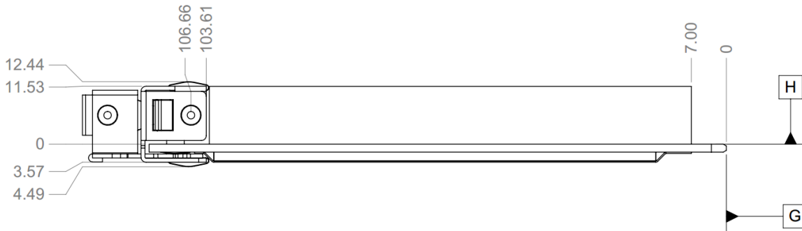
Figure 50: Large Form Factor OCP NIC 3.0 Card with Ejector CTF Dimensions (Side View)
