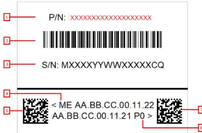
Figure 58: Baseboard MAC and Serial Number Label Example
