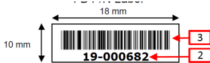
Figure 61: System Vendor Part Number Label Example
