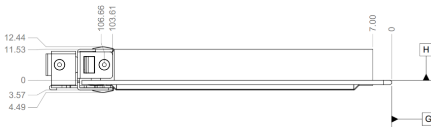
Figure 35: Large Form Factor OCP NIC 3.0 Card with Ejector CTF Dimensions (Side View)
