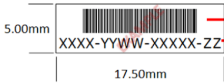
Figure 58: NIC Vendor Serial Number Label Example
