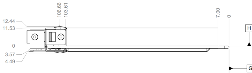
Figure 35: Large Form Factor OCP NIC 3.0 Card with Ejector CTF Dimensions (Side View)
