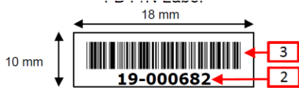
Figure 61: System Vendor Part Number Label Example
