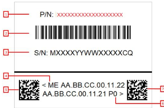
Figure 59: Baseboard MAC and Serial Number Label Example
