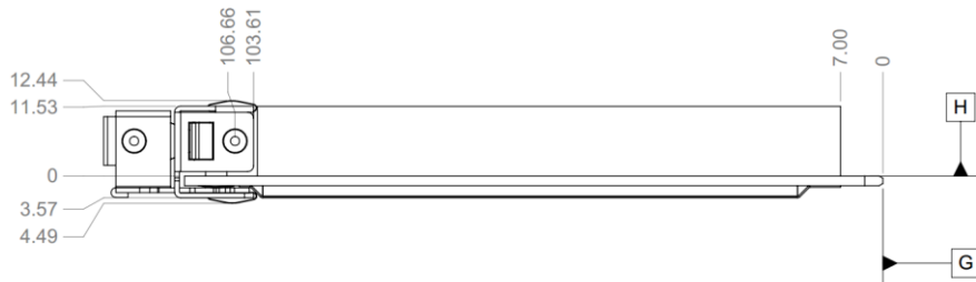
Figure 35: Large Form Factor OCP NIC 3.0 Card with Ejector Critical-to-Function (CTF) Dimensions (Side View—Left)
