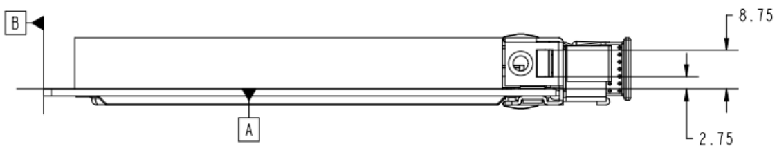
Figure 13: Small Form Factor OCP NIC 3.0 Card Critical-to-Function (CTF) Dimensions (Side View – Left)
