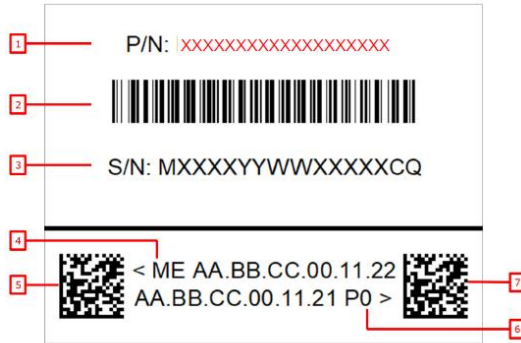
Figure 47: Baseboard MAC and Serial Number Label
