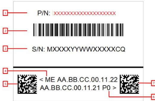
Figure 49: Baseboard MAC and Serial Number Label
