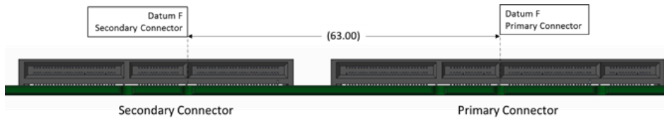
Figure 58: Primary and Secondary Connector Locations for Large Card Support For Right Angle Connectors
