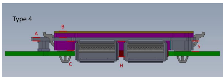
Figure 11: Type 4 Vertical Stack Front View
